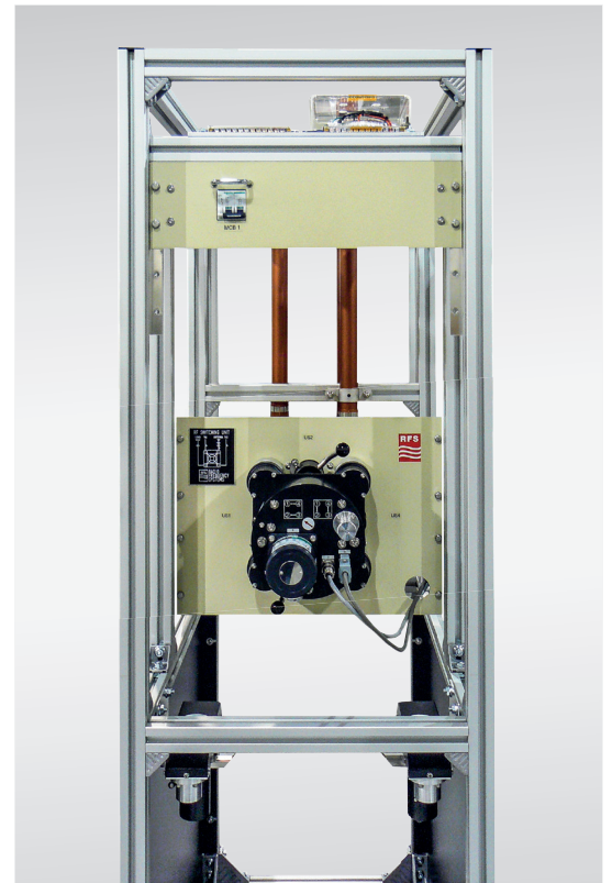
Switch frame featuring electrically operated coaxial switch and manual U-link back up for MMBI
