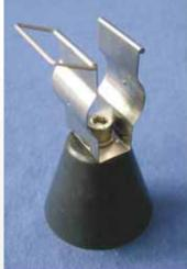
In case of fire the resistant part of the fixing will hold the cable in position and enables the cable to keep in operation as long as the cable itself allows. It also prevents the cable from detaching from the wall that might block any escape route.
